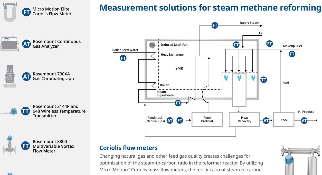
can be more easily and accurately maintained in real time. This is due to the mass ratio being more closely aligned with the molar ratio than it is with the volumetric ratio. Optimizing the steam-to-carbon ratio helps to extend catalyst life, decrease energy costs, and increase safety.
