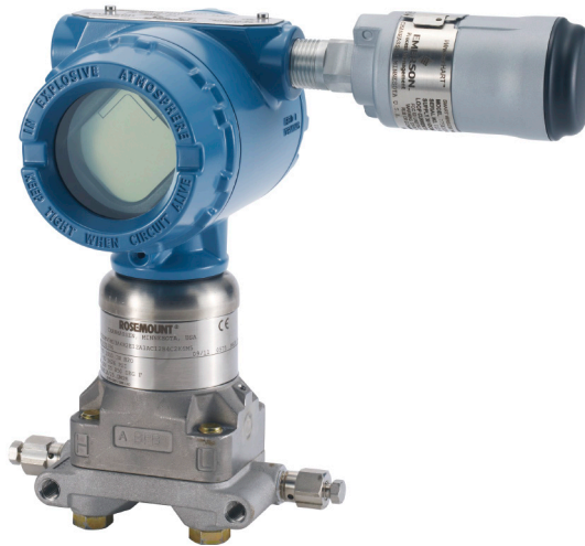
Figure 1.4: Emerson's Wireless 775 THUM™ Adapter can be added to HART enabled instruments with advanced diagnostics to send data and diagnostic information via a WirelessHART network.
