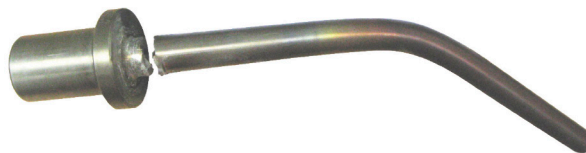
Figure 5.2: Severe vibration causes metal fatigue which can result in a break.
